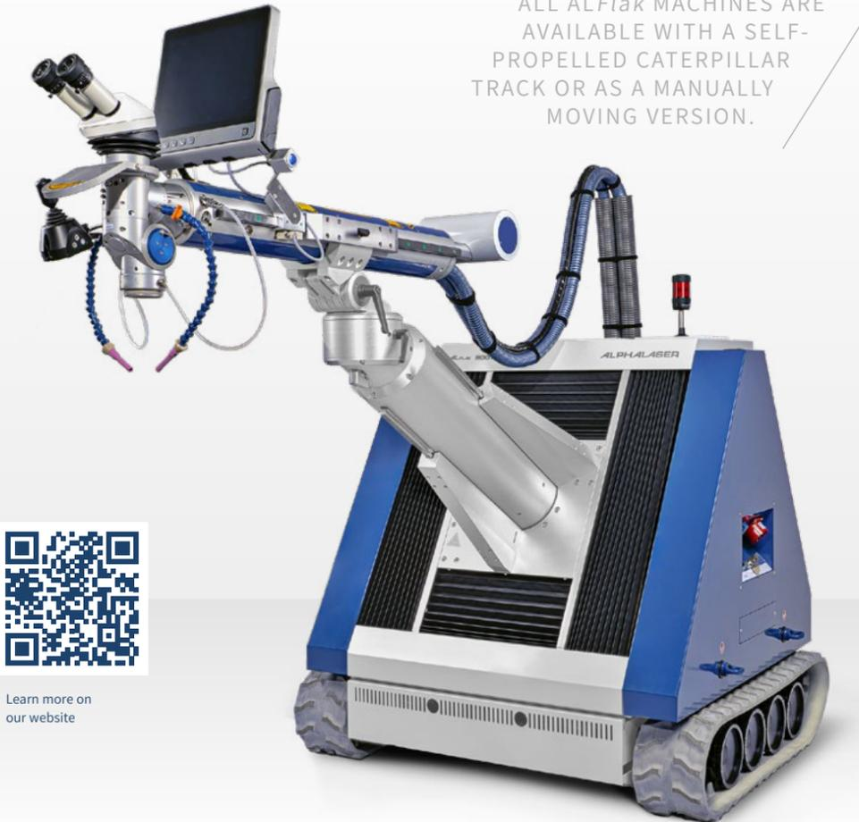
ALL ALFlak MACHINES ARE AVAILABLE WITH A SELF-PROPELLED CATERPILLAR TRACK OR AS A MANUALLY MOVING VERSION.
