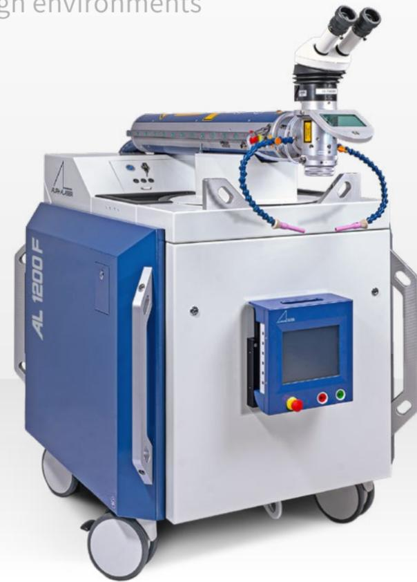
The ALPHA LASER 1200-Watt welding lasers are ideal for applications in the oil & gas sector, marine shaft repair, hard facing with wire and powder, in hydroelectric power plants (casting repairs) and for large but sensitive components where TIG welding becomes problematic. The laser systems are also suitable for mobile use or as a stationary workplace in the workshop.
