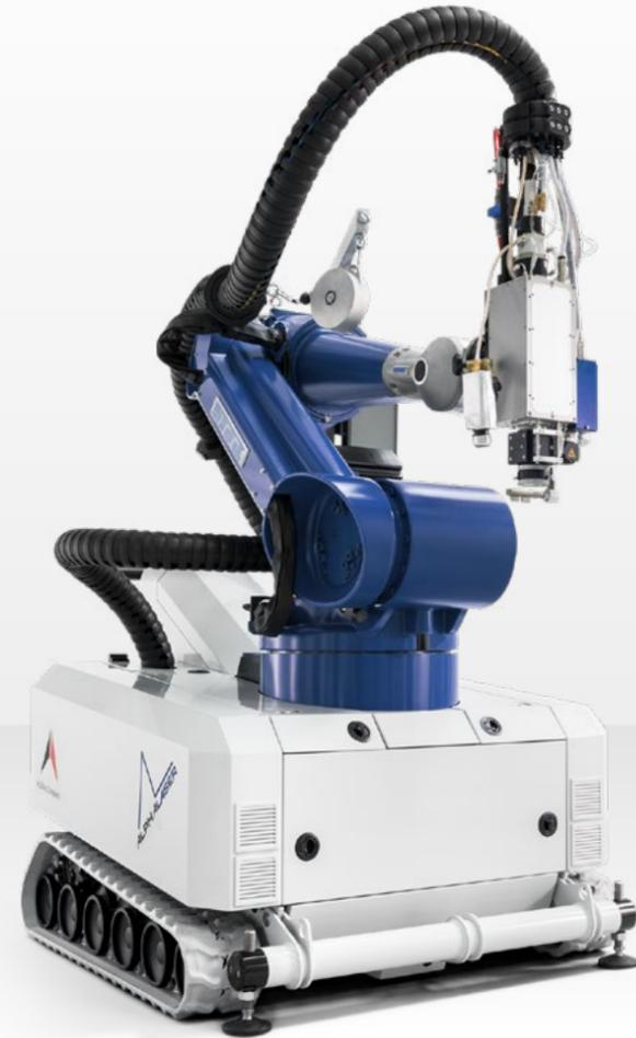
The **AL-ROCK MOBILE (our MINI-ROCK)** is the first truly mobile robot for the targeted laser hardening of metal surfaces. All components such as laser source, optics, control, cooling, powder feeder and safety technology are integrated in the system.
